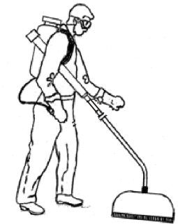
Place the backpack tank on the operator's back and connect to the HANDYDOME
