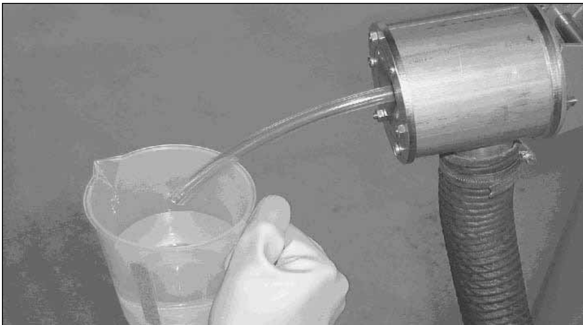
Fig. 4 – Tube Fitted to Sprayhead for Calibration
